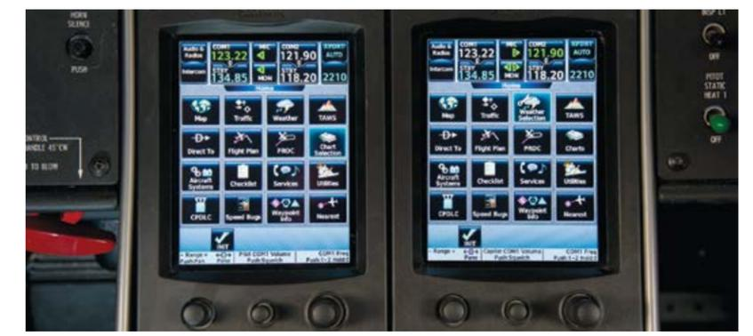
The GTC 570, an all-new glass touch-screen controller, is the primary connection for the Garmin G3000 system. This icon-driven interface enables you to access more systems and sensors than ever before. Functions are easy to locate with fewer touch points, allowing you more time heads up, looking forward.
