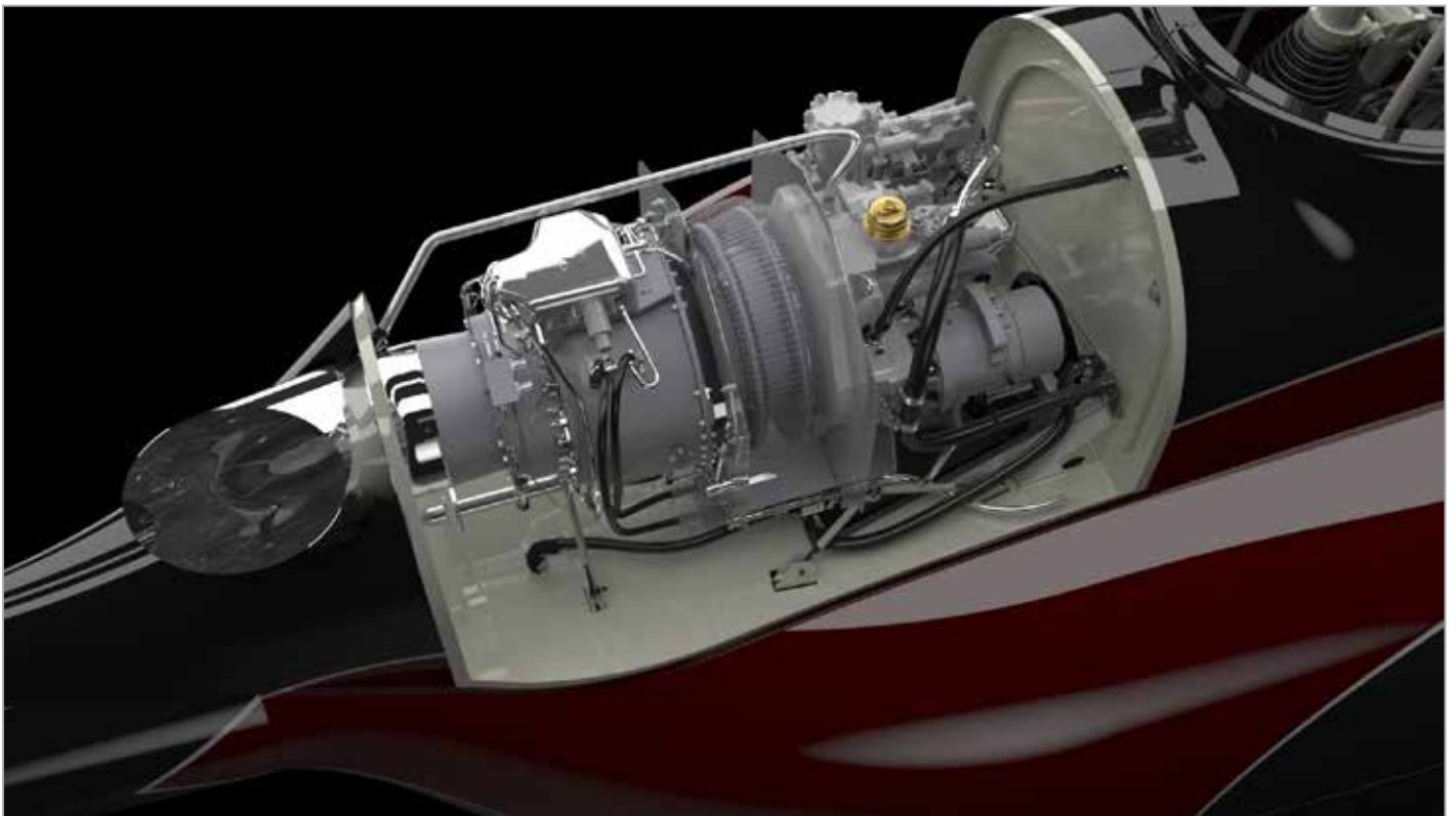
The Bell 505's Safran Arrius 2R Engine features a dual channel FADEC with automatic backup.
