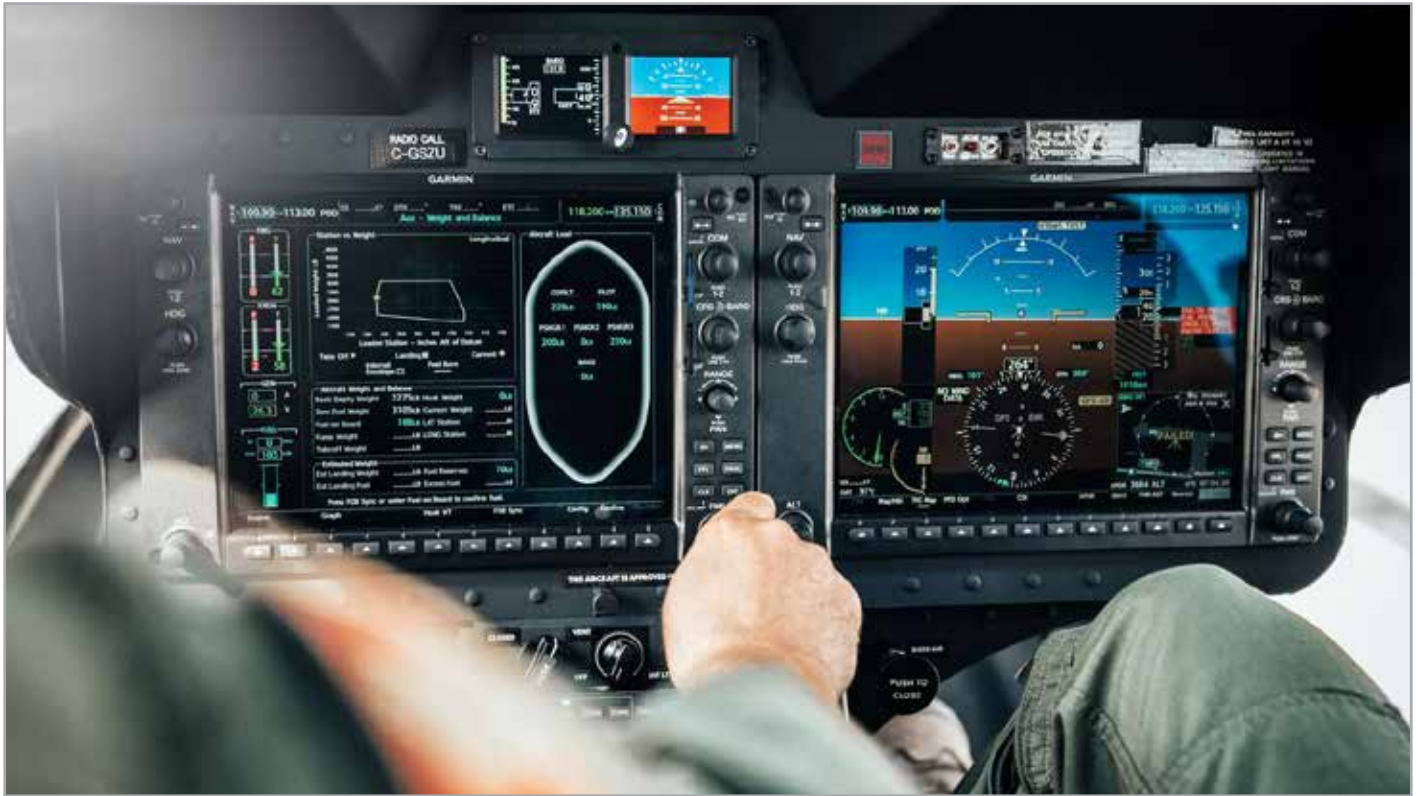
The Bell 505 Garmin G1000H NXi Flight Deck provides the next level of safety.
